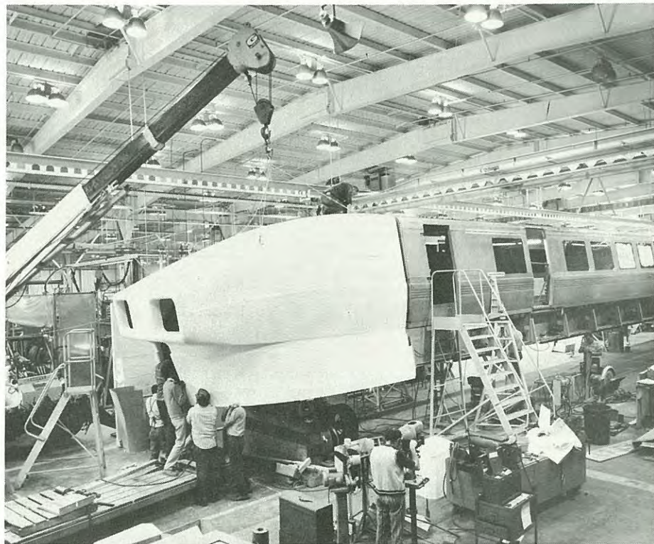
Figure 2-6. Positioning Forebody for Installation
